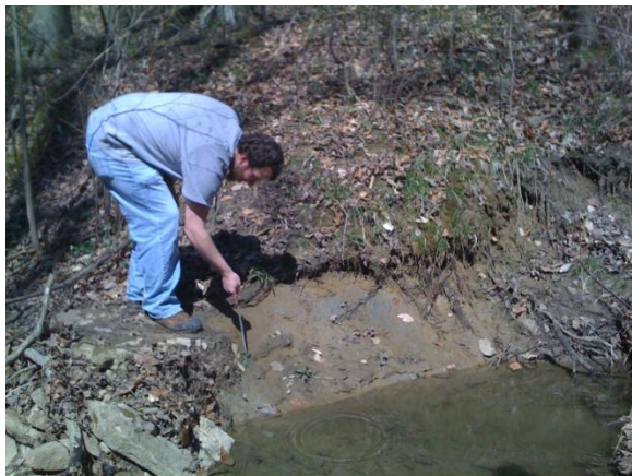
Figure 8: On the opposite side of the valley where the Lawyers Pt. landslide occurred was a stream that had exposed lakebed clays seen here in their dark grey and blue (Photo by Sarah Johnson).
