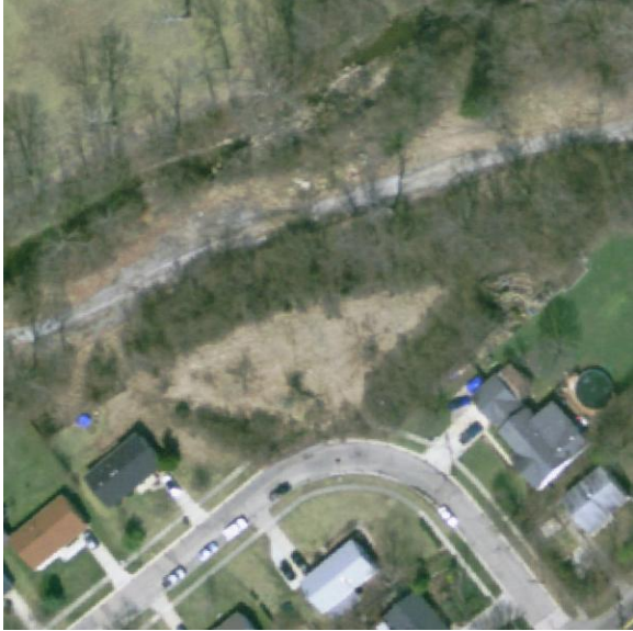
Figure 16: Aerial photograph obtained from the OSIP aerial imagery archive of the landslide located off of Huffman Ct. north of Cincinnati, OH. The top of the slide can be seen affecting the sidewalk on the northeast side of the turn in the road. The gray feature near the bottom of the slide is an access road which is moving with the slide.
